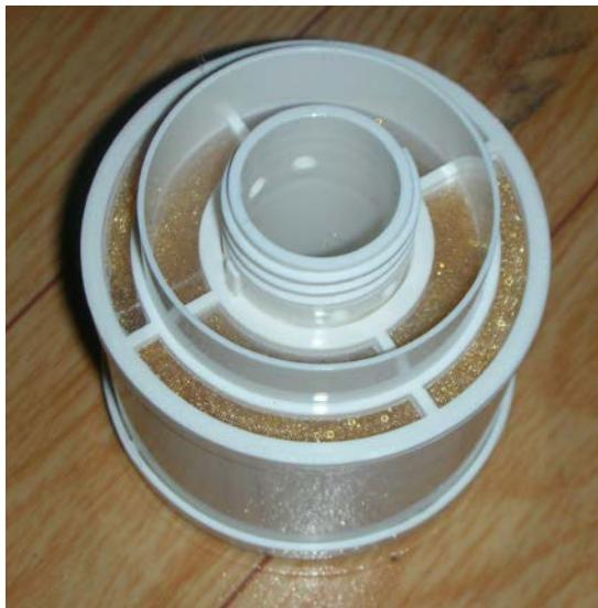
The water filter in your device is black , however - to increase the visibility of the ion-exchange resin - here a white filter.
