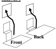
Insert the rear pin into the stamped hole on the cabinet wall
