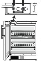
**19.** Insert the bottom hinge pin in the same way.
