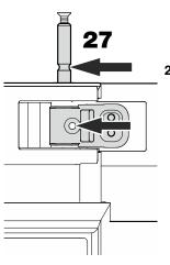
**27.** Push in hinge pin until groove in the pin lines up with bore hole in the hinge bracket.
