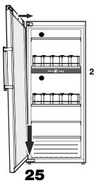
**25.** Place door on pin and move the top of it to the hinge bracket.
