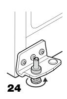
**24.** Insert pin fully into hinge bracket and tighten adjustable foot by hand.
