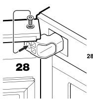
**28.** Undo screw in hinge pin and screw into bore hole in hinge bracket.
