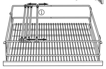
Lock the bottle holder in the required position on one of the support bars.
