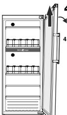
4. Tilt door slightly to the side and remove by lifting upwards.
