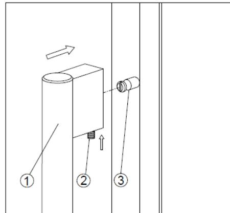
Locate the handle (1) over the pins (3) of the door and tighten the handle by screwing the allen key grub screws.
