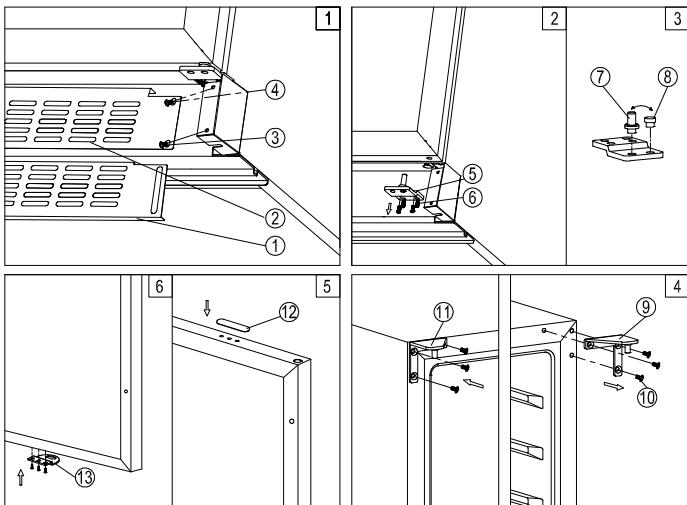
1. Remove the ventilation grille ② and the adjustable ventilation grille ① by unscrewing the screws ③ & ④. (Fig. 1)
