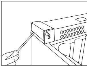
4. Carefully remove the covers on the side of the plinth using a flat-headed screwdriver.
